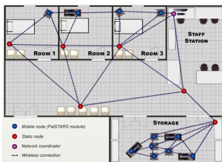
Figure 3: Example PatSTARS network configuration
