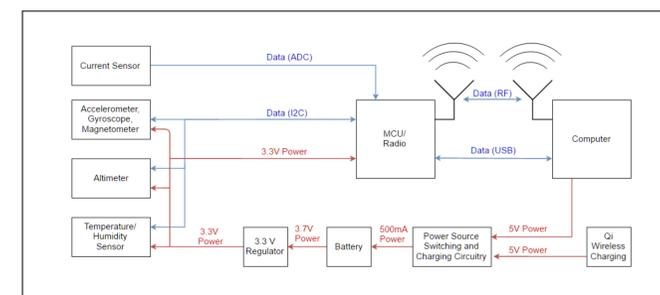
Figure 2: PatSTARS module block diagram
