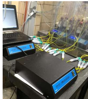
Figure 3. Respirometers attached to batch test set-up
