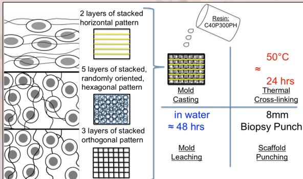
**Figure 1.** Schematic representation of cellular alignment of cartilage with corresponding schematics of scaffold molds and flow chart representing the investment casting process.
