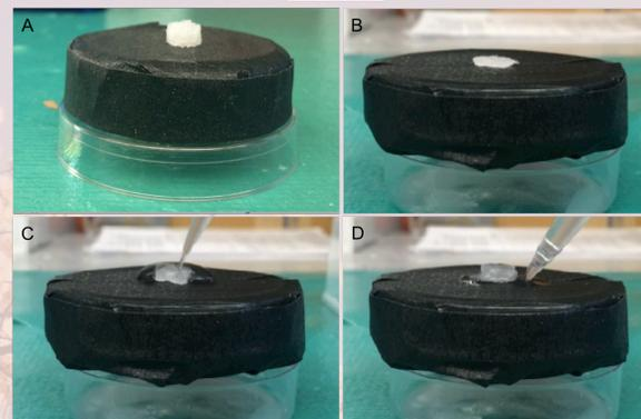
**Figure 2.** Time-lapse images of the shape memory response of the scaffolds. (A) Undeformed scaffold; (B) Deformed scaffold; (C) Scaffold mid-recovery; (D) Fully recovered scaffold.
