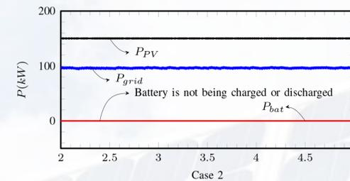
Stop charging the battery, switch PV to **reference power control mode** to balance power flows.
