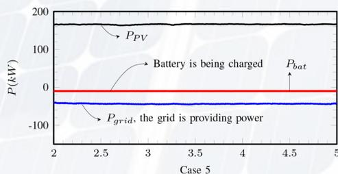
Request power from the main grid to balance the power and charge the battery.
