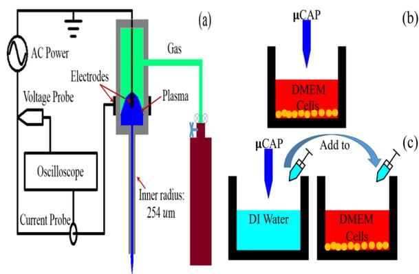
**Figure 2.** (a) Schematic representation of micro-sized cold atmospheric plasma setup. (b) Micro-sized cold atmospheric plasma ( $\mu$ CAP) direct treatment:  $\mu$ CAP directly treated DMEM containing cells. (c)  $\mu$ CAP indirect treatment:  $\mu$ CAP treated DI water and remove it to DMEM containing cells (70% DMEM + 30% treated DI water).
