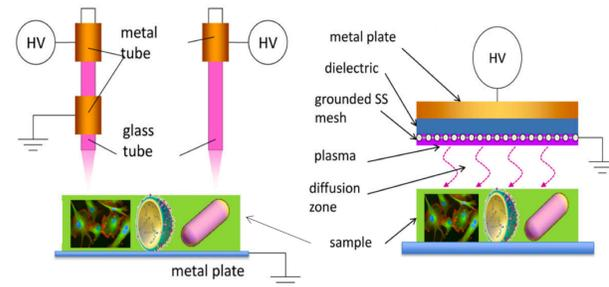
**Figure 1.** Sketch of indirect plasma jet and DBD configuration with sample treated
