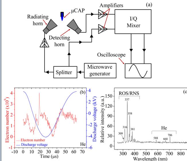
**Figure 3.** (a) The schematics of Rayleigh Microwave Scattering System (RMS) experimental setup, (b) electron number per period discharge of He  $\mu$ CAP ( $2.4 \times 10^9$ ), and (c) Optical emission spectrum detected from the He  $\mu$ CAP using UV-visible-NIR.
