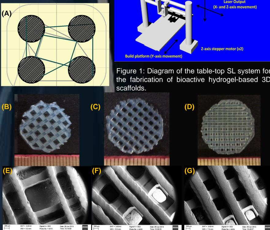
Figure 2: (A) 2D CAD model. Photo and SEM images of 3D printed porous hydrogel scaffold via our novel table-top SL apparatus with (B)-(E) 40%:60%; (C)-(F) 60%:40%; and (D)-(G) 80%:20% fill density/porosity.
