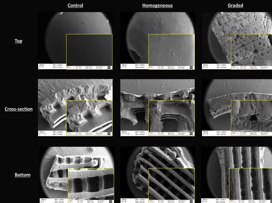
Figure 3: Scanning electron micrographs of SL 3D printed bioactive nanocomposite PEG-da osteochondral scaffolds.
