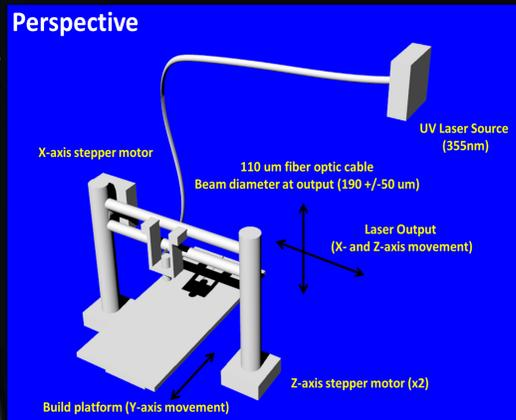
Figure 1: Diagram of the table-top SL system for the fabrication of bioactive hydrogel-based 3D scaffolds.
