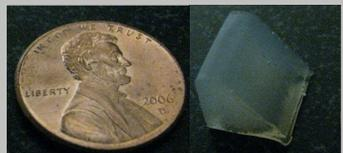
Figure 1.3 - Silicone Self-Oscillating VF Model
