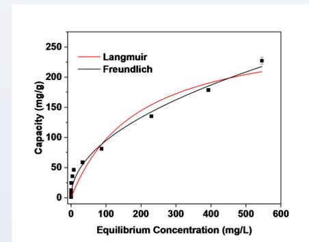
The product has an impressive adsorption capacity of near 200 mg/g.
