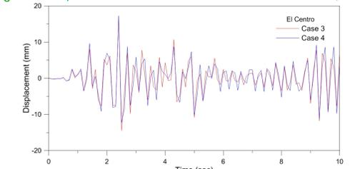
Figure 7. Displacement of the structure under El Centro record for cases 3 and 4 with 5% of damping.
