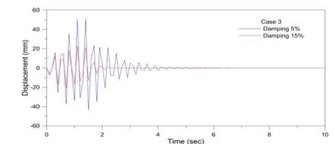
Figure 6. Displacement of the structure under sinusoidal motion (a=0.30g).
