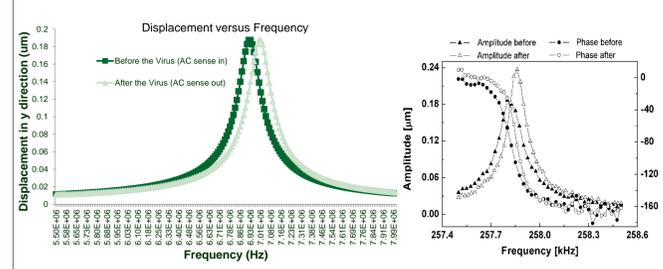
The frequency change can be sensed by using the Spectrum/Signal analyzer. Displacement/amplitude represents the average capacitance value between the resonator and the sense electrode during the oscillation. The graph on the left side shows an example result from the Coventor Simulation and the graph on the right side shows an example from the real results published in [3]
