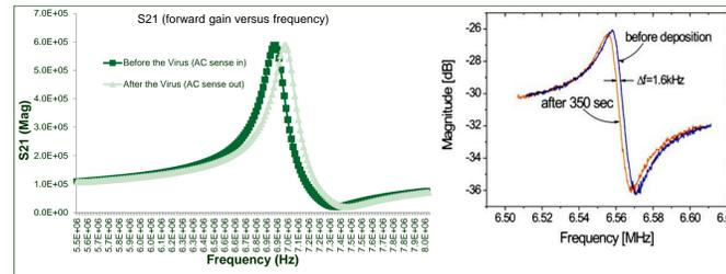
The frequency change can also be sensed by using the Network analyzer. S21 represents the forward gain by taking into account the capacitance value between the resonator and the sense electrode during the oscillation. The graph on the left side shows an example result from the Coventor Simulation and the graph on the right side shows an example from the real results published in [4]
