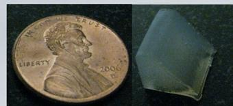
Figure 1.3 - Silicone Self-Oscillating VF Model
