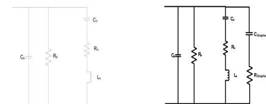
(a) Equivalent Circuit for bare dipole
