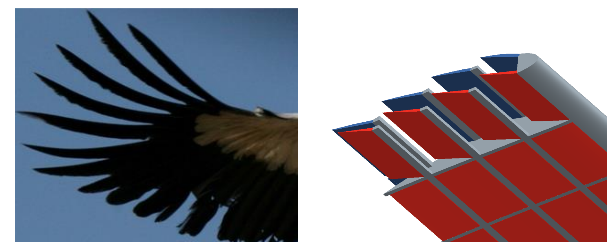
Figure 3: The splayed profile of an avian wing (left) and bioinspired wing (right)
