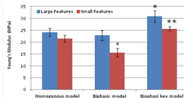
Figure 3. Figure 24; Young's modulus data for 3D printed scaffolds. Data are  $\pm$  SEM, n=5; \*p<0.05 when compared to all homogenous and biphasic scaffolds; \*\*p<0.05 when compared to all other scaffolds with small features; and #p<0.05 when compared to all other scaffolds.
