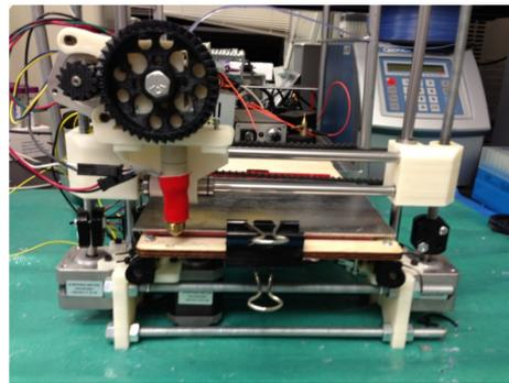
Figure 1 The lab's FDM 3D printing setup
