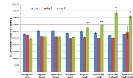
Figure 4, MSC proliferation in a variety of 3D printed PLLA scaffolds with different internal structure and surface modification. Data are  $\pm$ SEM, n=9; \*p<0.05 when compared to all other scaffolds and \*\*p<0.05 when compared to all scaffolds with large features and homogenous controls with small features at day 5.
