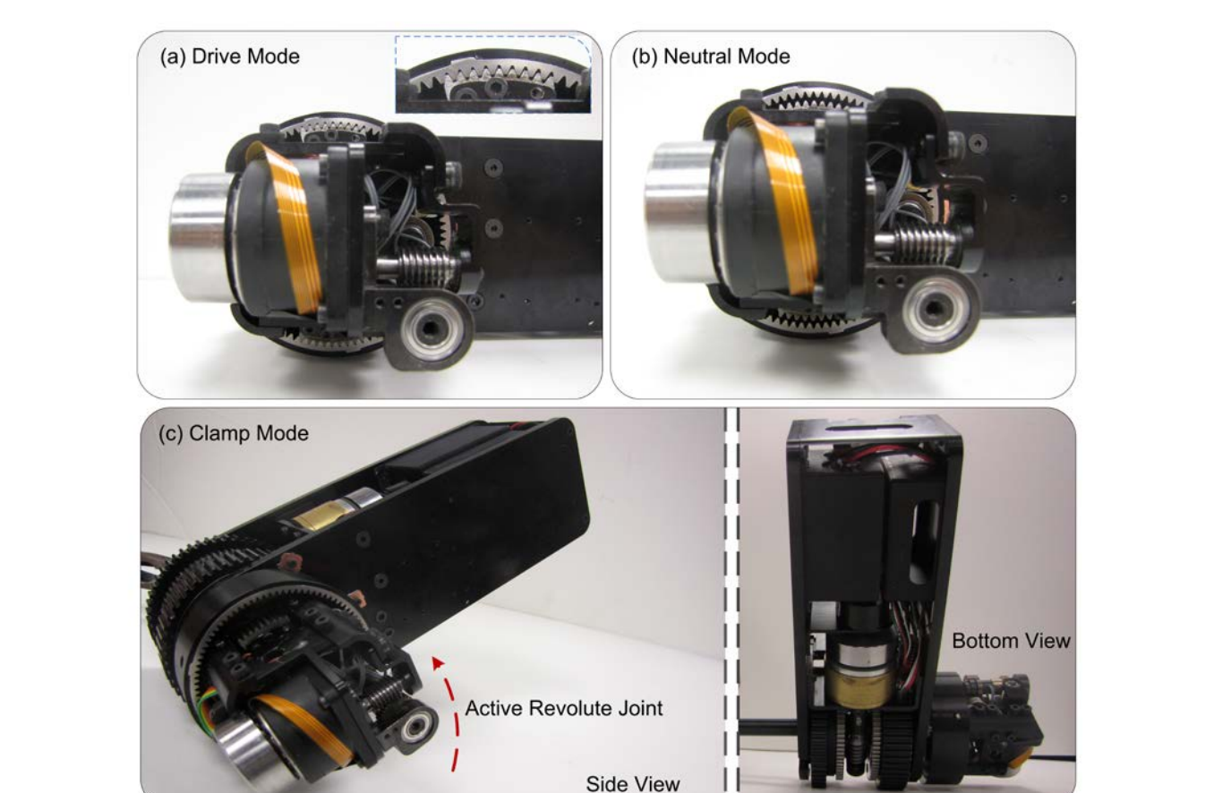
Figure 9: Prototype of the docking interface connected to a small mobile robot, with details showing the drive, neutral and clamp modes
