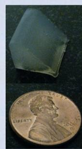
Figure 1.4 - Silicone Self-Oscillating Vocal Fold Model
