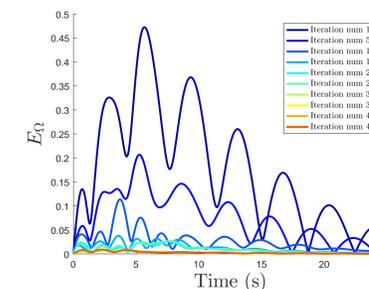
Figure 5: Angular velocity error  $\|\Omega_{z,k} - \Omega_k\|$
