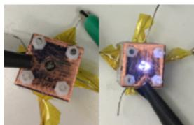
Figure 1. Matrix Thruster Head Non-firing and Firing with 4 Cathodes Energized
