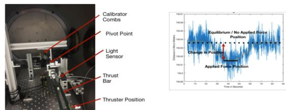
Figure 4. Stand (Left) and Measured Step Data (Right)
