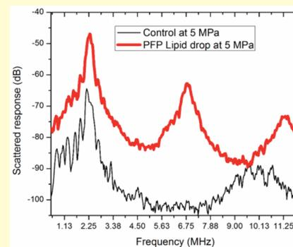
At high excitation pressure, scattering signals from the vaporized nanodroplets were significant. This figure shows acoustic responses of vaporized droplets at 5 MPa with 2.25 MHz center frequency.
