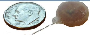
Figure 1: Previous generation of miniature pacemakers. Our lab previously developed a wireless implantable pacemaker for mice (Laughner et al., 2013).
