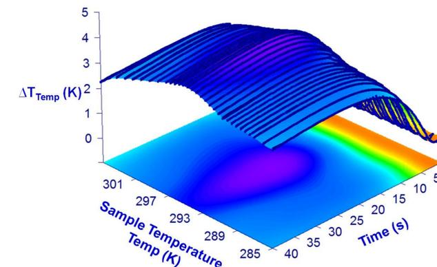
3D surface plot of Gadolinium  $\Delta T_{Temp}$  curve,  $\Delta T_{Temp}$  as a function of Sample Temperature, Time and Applied Field.
