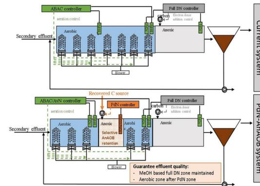
Intermittent Aeration → Aerobic DO concentration: 1.5 mg O<sub>2</sub>/L
